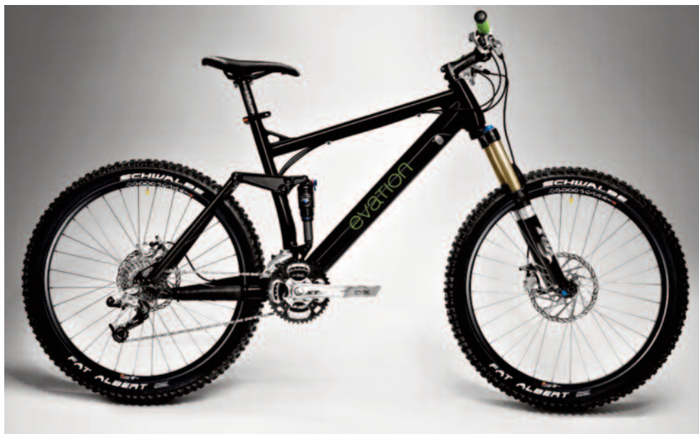
FAZUA's patented evation electric drive system is compact, lightweight, and removable. Its components blend into the bicycle frame and are all but invisible except on close inspection. (Photo by Stefan Schmalzgruber)
