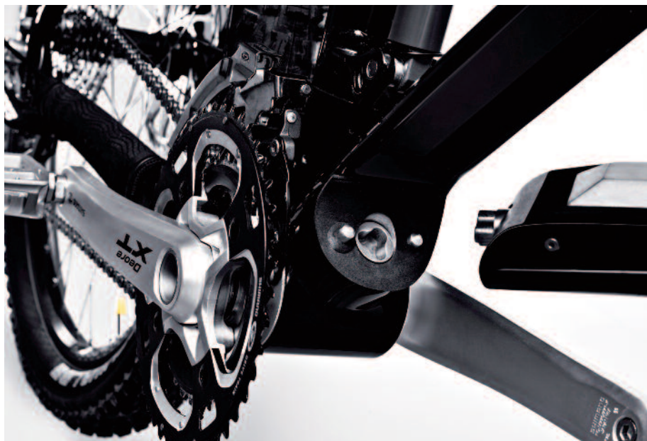
A driveshaft connector with a precisely designed polygon profile connects the motor and transmission in the evation design. One end of the drive packet slips into it with a simple click. (Photo by Stefan Schmalzgruber)
